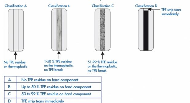
The second character describes if the TPE strip will tear during the measurement at any position on the peel path.
